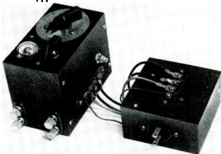
The bridge (left) is shown with its selenium-rectifier power supply.
